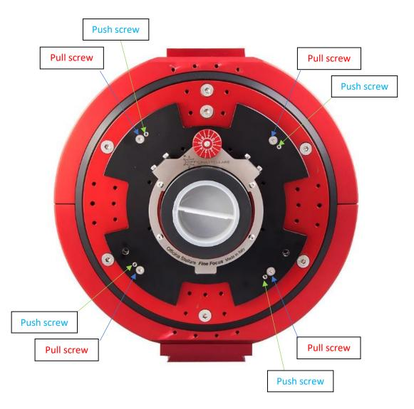
Work with only on one screw at a time. Then take an image, check the corners, and adjust other screws or stop. Use the push screw to gently lock the pull screw.
