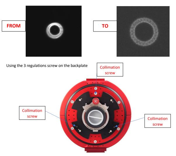
Now you have the telescope collimated, it's time to take some images to check the rest of the system. You need to take one image at focus and another just a little bit out of focus.
