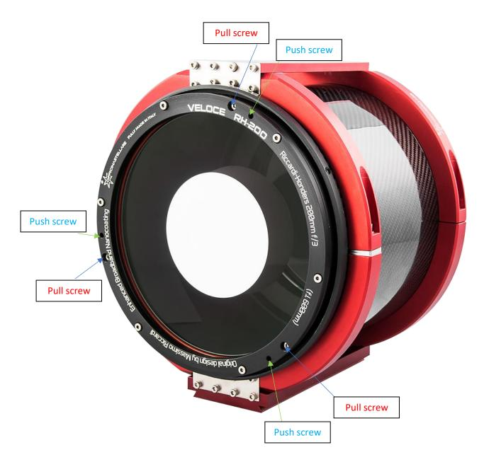
Under the pull screws (blue arrow) there are cup springs to keep collimation. If these screws are/or become too tight, you need to unscrew them. Start by unscrewing all pull screws 1 turn. This will reduce compression on the front lens cell from the cup springs. Then take another image to see if the star's shape has changed.
